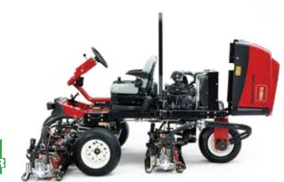
A simplified tractor design utilizing a Tier 4 compliant engine, without the expense or complexity of larger engines that require Tier 4 after-treatment systems, saves money in fleet maintenance expenses.
